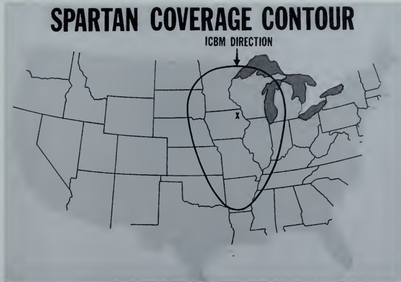
Fig. 2-15. Elliptical footprint of the area covered by a SPARTAN missile system from a hypothetical base in Iowa.
